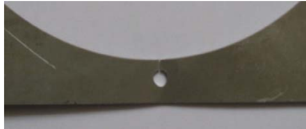
Fig. 6 - Cutting entry point close-up
