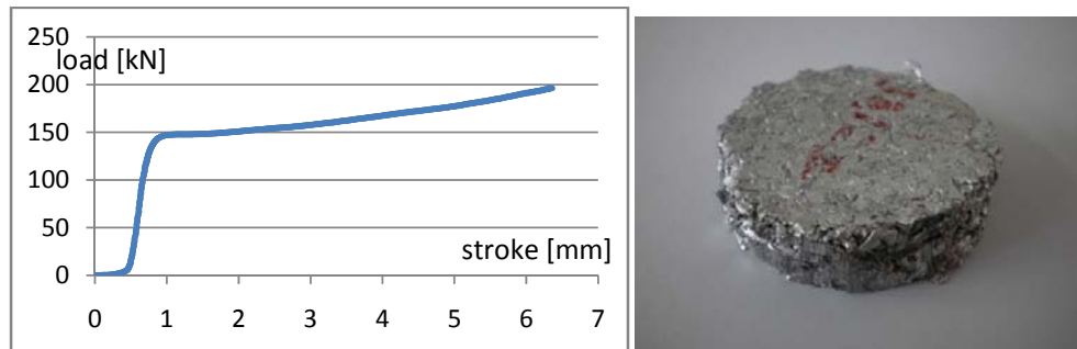
Fig. 7 – Load–stroke diagram and workpiece after free upsetting
