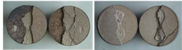
Fig.11. The aspect of samples fracture surfaces, with 6 deposited layers achieved by HVOF thermal spraying process of WOKA 7504 powder, after performing adhesion tests: a) \varnothing 25 mm sample, S235JR substrate; b) \varnothing 25 mm sample, 304L substrate
