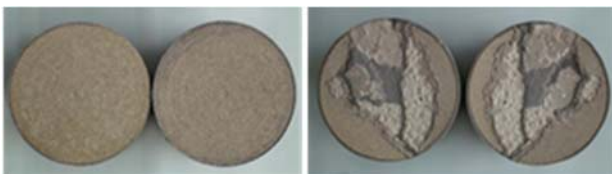
Fig.10. The aspect of samples fracture surfaces, with 4 deposited layers achieved by HVOF thermal spraying process of WOKA 7504 powder, after performing adhesion tests: a) \varnothing 25 mm sample, S235JR substrate; b) \varnothing 25 mm sample, 304L substrate
