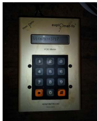
Fig. 9 Electronic clock for measuring of velocity of detonation
