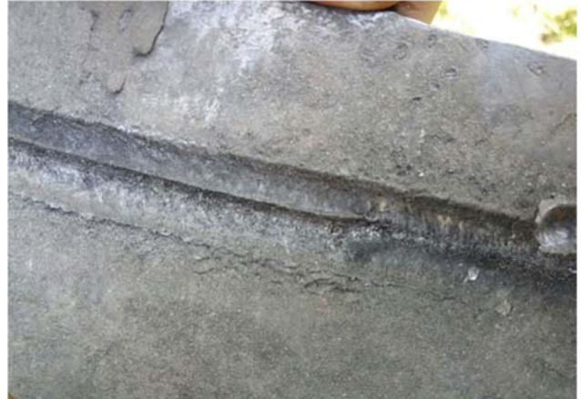
Fig. 7 Formed notch after the detonation
