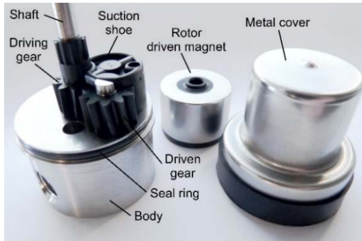
Fig. 1. Disassembly of the magnetic drive micropump
