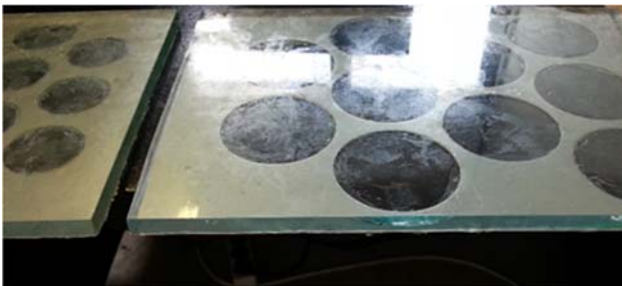
Fig. 1. Small scale models of the hybrid elements representing its structure (glass – adhesive – steel)
