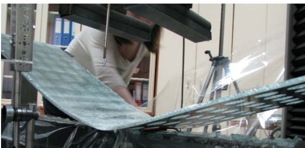
Fig. 4. Full hybrid element failure
